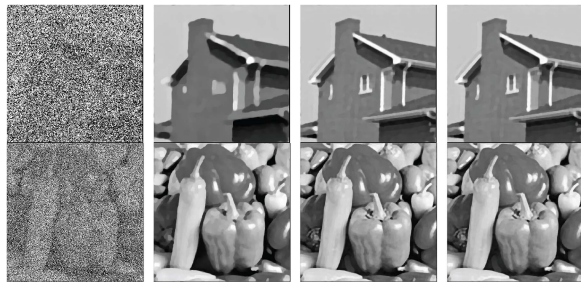
Fig. 2. Visual results for images corrupted by Gaussian blur with 70% SP noise and restored by TVL1, TVSCAD, and NNDCL1.
