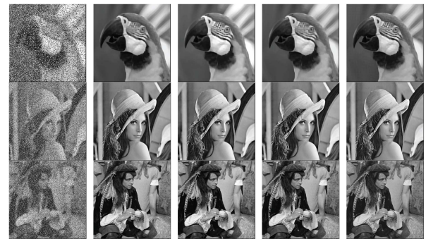
Fig. 9. Average blur image with 30% SP noise and images restored by ETTV, L0TV, NNADM, and NNDCL1.
