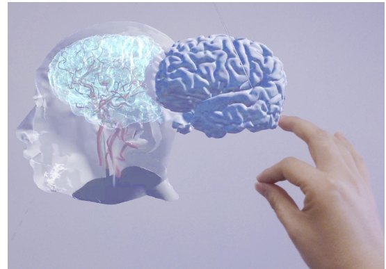
Fig. 7. An operation of dragging the white matter out from the digital brain through a pinch of the right thumb and the index finger. The skin and the gray matter are made fully transparent by two sliders.
